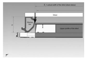
The ideal measurements of the blind are in the diagram. Such measurements can be taken by using the cut of the upper profile; by the aid of the side board place on the glazing bar, it is possible to record the point, the maximum possible width of the blind. From this point the dimension of the same point on the opposite side is measured. This marking is always influenced by the form and size of the glazing bar of the window profile.
