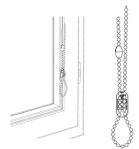
APPLY ONE HALF OF THE COUPLER TO EACH END OF THE CHAIN AND THEN LOCK BOTH COUPLER HALVES.
